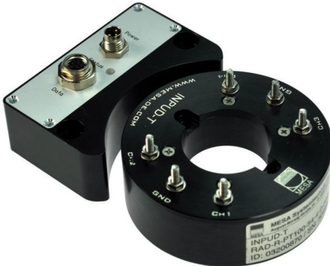
INPUD-T (Inductive Power and Data Transmission) is a compact system for contactless transmission of Pt100 transducers. INPUD-T is able to transmit two or four channels simultaneously.
